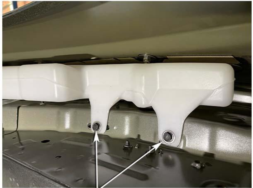
Standard M6 Bolts with M6 x18 Body Washers Installed
