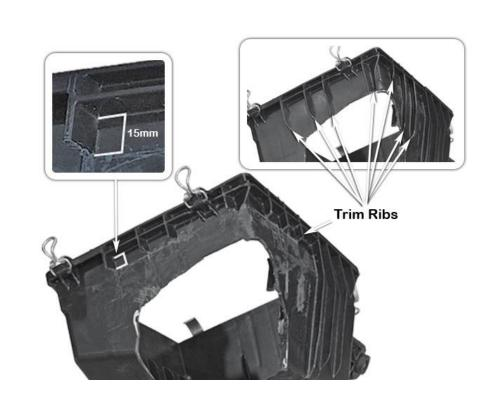
Align the Side Air Cleaner Template (Item 20) to the air cleaner base as shown.
