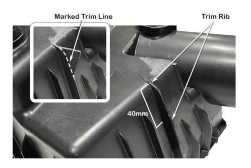
Mark the air cleaner base around the edge of the standard air inlet snout where shown.
