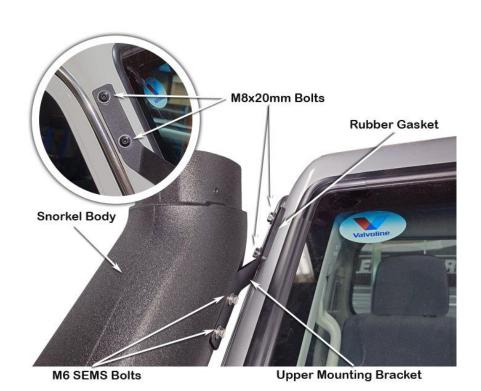
Install the ARMAX air ram assembly (Item 2) onto the snorkel body.
