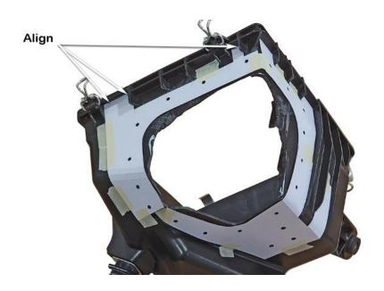
With all three templates aligned on the air cleaner base, mark all 20 hole positions and the required air cleaner base cut-out.
