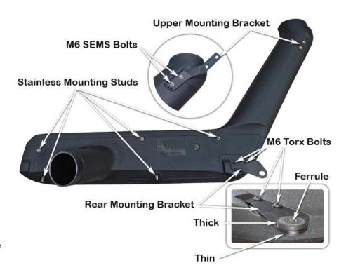
Apply Loctite 243 to the two M6 x 12mm Torx bolts (Item 7) and secure the Rear Mounting Bracket (Item 5) to the Snorkel Body (Item 1) as shown.
