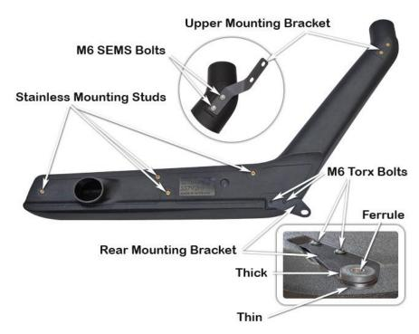
Apply Loctite 243 to the two M6 x 12mm Torx bolts (Item 8) and secure the rear mounting bracket (Item 7) to the snorkel body (Item 1) as shown.
