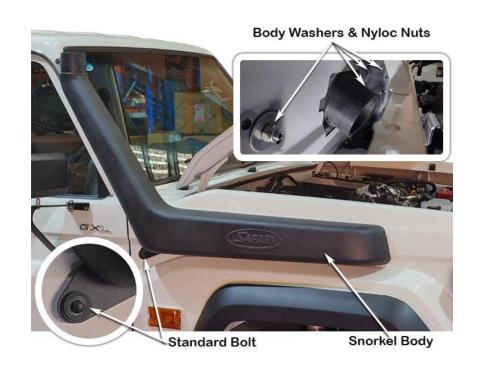
Secure the upper mounting bracket (Item 3) to the A 'Pillar using the x2 20mm long genuine Toyota A-pillar bracket mounting bolts retained in Step 2.
