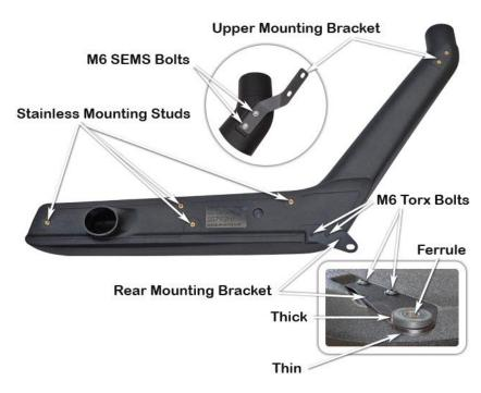
Apply Loctite 243 to the two M6 x 12mm Torx bolts (Item 8) and secure the rear mounting bracket (Item 7) to the snorkel body (Item 1) as shown.
