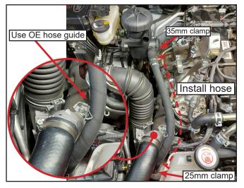
Install the supplied **short hose** to the breather port on the rocker cover using **25mm spring clamp (item 11)**, then connect the silicone expander end to the upper port of the oil separator using a **35mm spring clamp (item 10)**.
