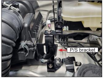
Adjust the oil seperator outlet orientation as shown.
