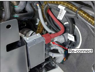
Install water sensor patch loom.
