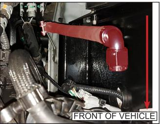
Install pre-filter to filter housing and connect the water sensor from patch loom to the new pre-filter assembly.
