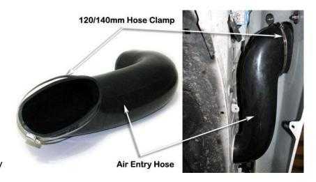
13 Install the 100/120mm hose clamp (Item 12) loosely over the outlet end of the air entry hose (Item 11). Install the air cleaner base into position whilst guiding the air cleaner base inlet snout into the air entry hose (Item 11). Secure the air cleaner base with the original mounting hardware. Align the air entry hose (Item 11) for best fit and tighten the hose clamps (Items 12 & 13) at each end of the air entry hose. Install the air cleaner element, air cleaner lid and any plugs or
