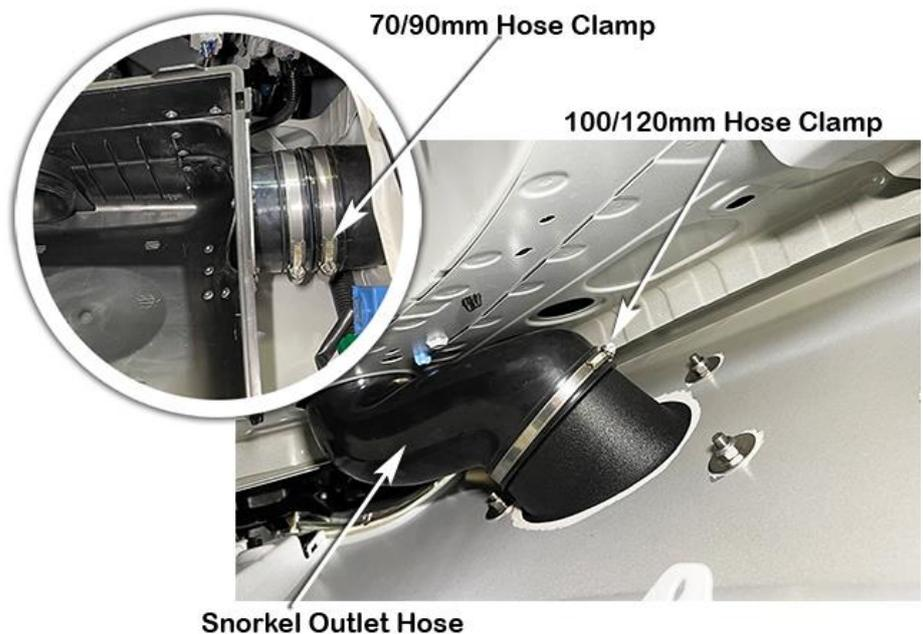
Loosely install the black hose clamp (Item 23) over the base of the air ram assembly (Item 2).
