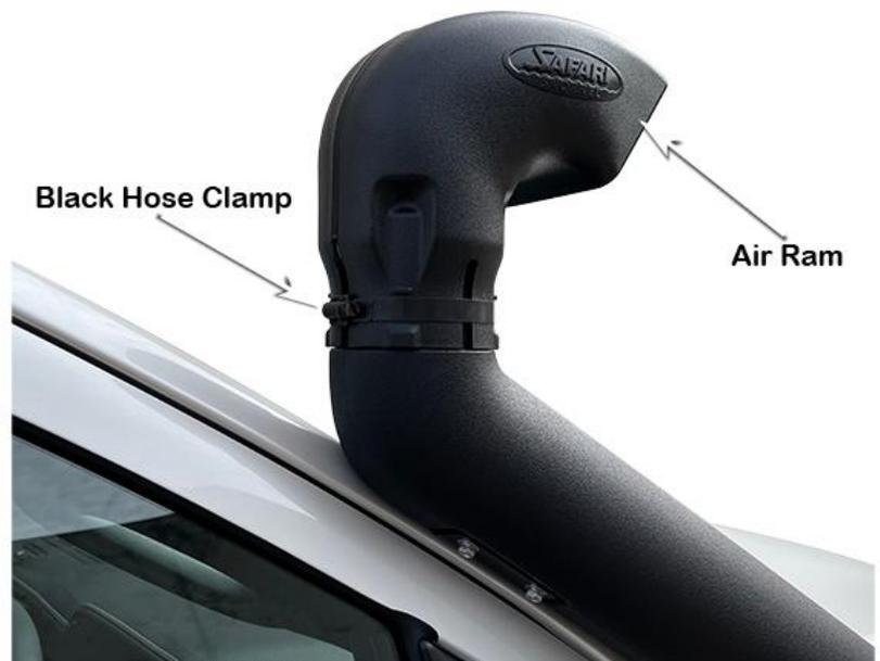
Install the RHS guard liner, mud flap, air cleaner element, air cleaner lid, reconnect sensor wiring and any other items that may have been removed during the snorkel installation process.
