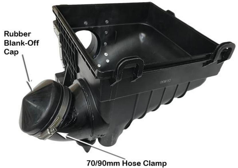
Install the stainless steel joiner (item 12) into the air entry hose (item 11), install a 70/90mm hose clamp (Item 21) onto the air entry hose and tighten.
