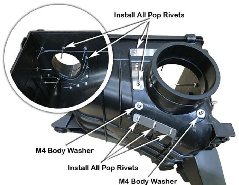
With the air entry hose, pop rivets and hose support plates correctly installed, secure all the pop rivets using a pop rivet gun.
