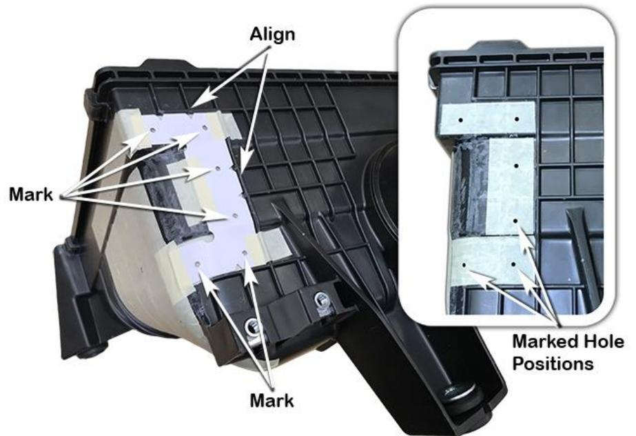
Drill a pilot hole for each of the seventeen marked hole positions, drill each hole position to 4.5mm diameter with a 4.5mm drill bit.
