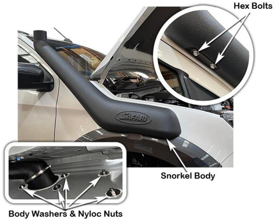
Ensure the snorkel outlet hose is correctly installed onto the snorkel body outlet and tighten the 100/120mm hose clamp (item 22).
