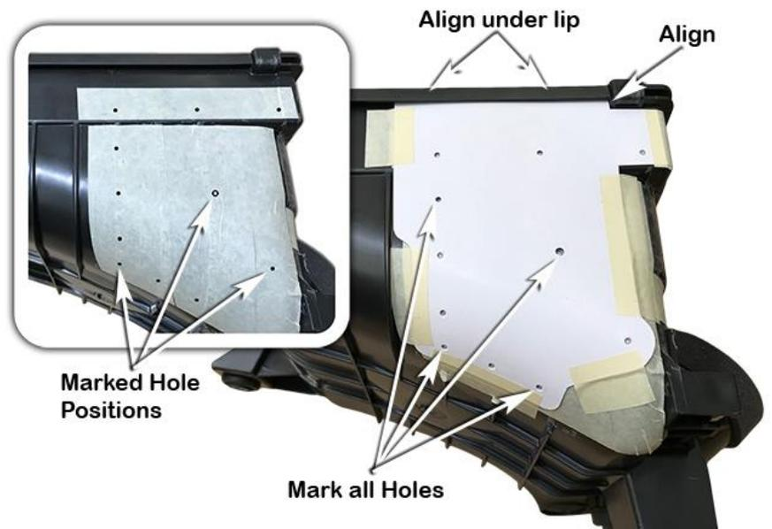
Align and tape the front air cleaner template (item 17) to the upper and side ribs of the air cleaner base as shown.
