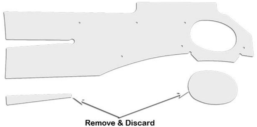
Align the guard panel template (Item 25) with the upper corner, upper and rear edges of the RHS guard panel as shown.
