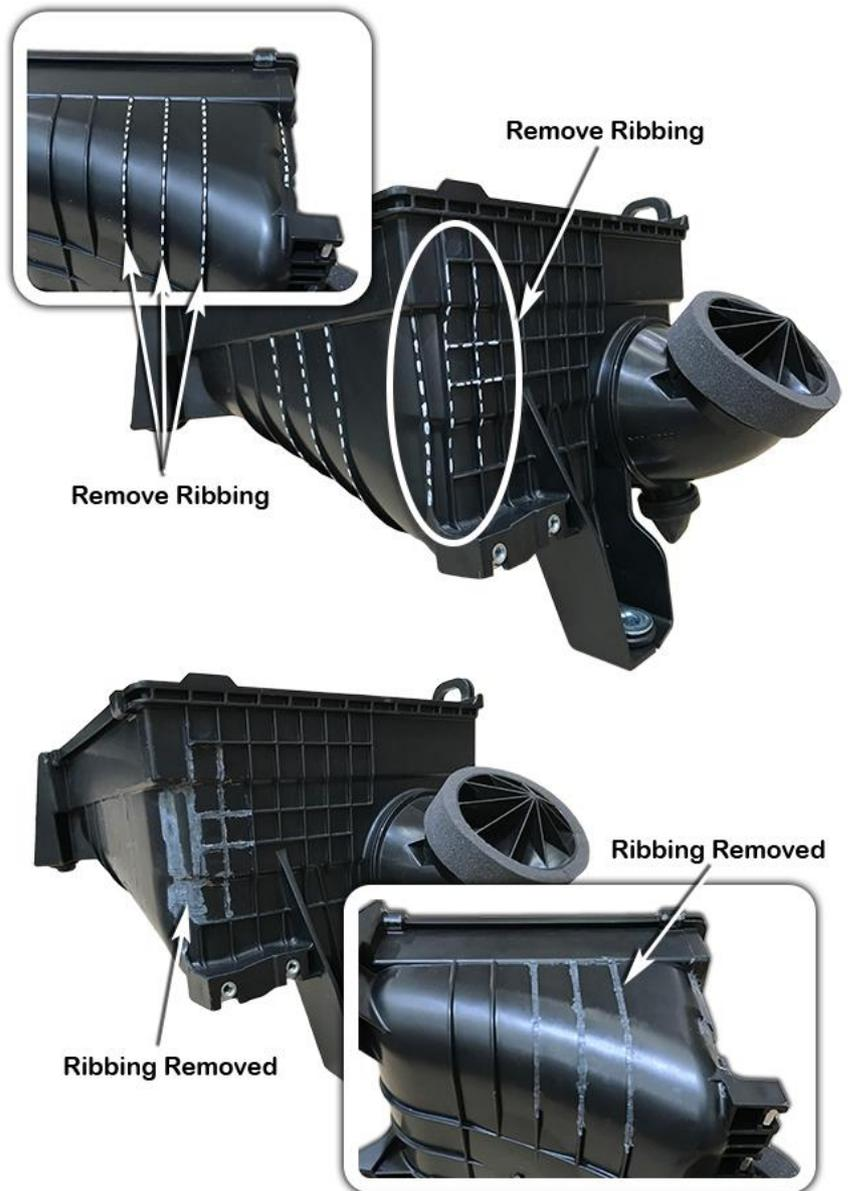
Remove the two internal ribs as shown.
