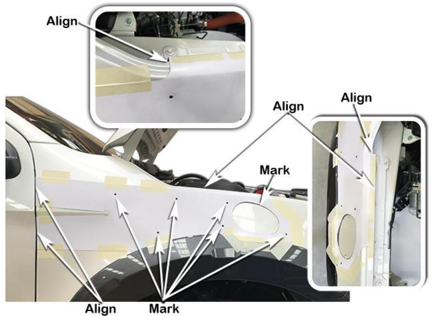
Drill a pilot hole for each of the marked hole positions.
