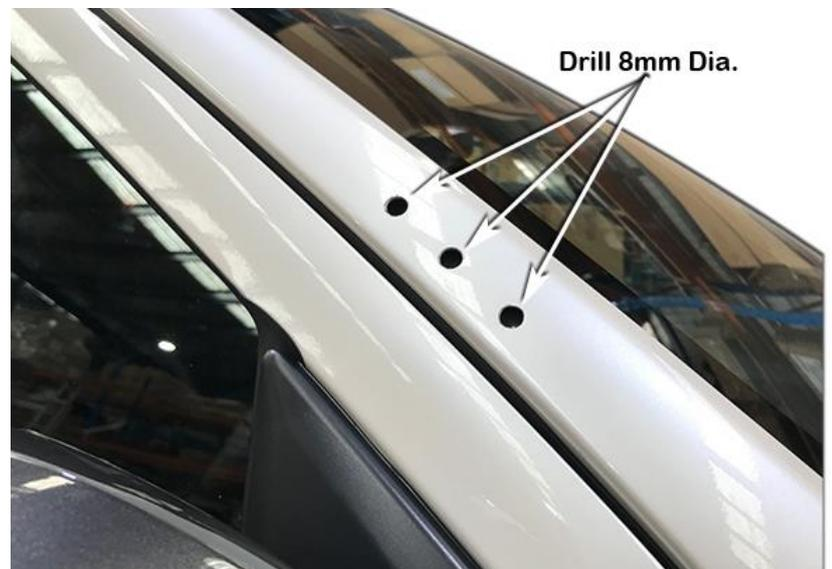
Install the plastic inserts (Item 6) into the 8mm diameter holes in the A-pillar.
