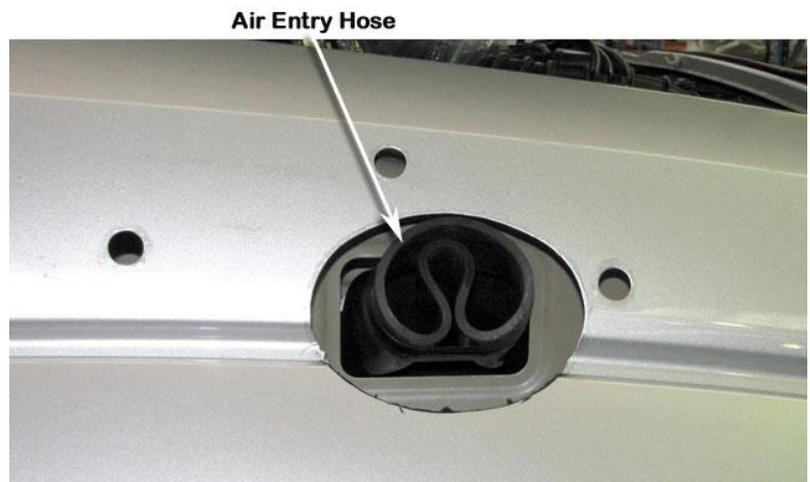
Shape the 90/110mm hose clamp (item 15) to the oval shape of the air entry hose, loosely install the hose clamp onto the air entry hose.
