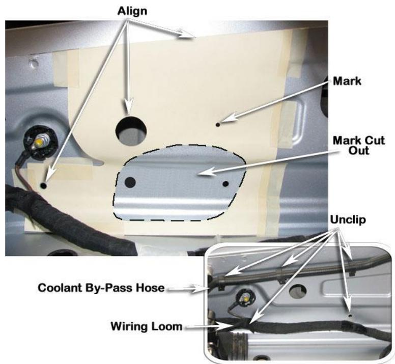
Drill a pilot hole at the marked hole position.
