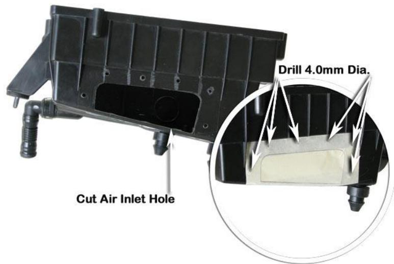
Place a strip of masking tape along the bottom of the air cleaner housing as shown.
