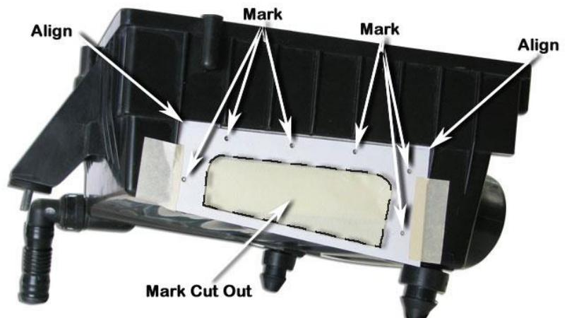
Drill a pilot hole for each of the marked hole positions.
