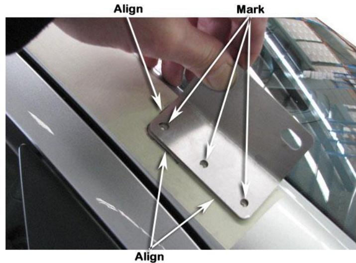
Drill a pilot hole at each of the three marked hole positions.
