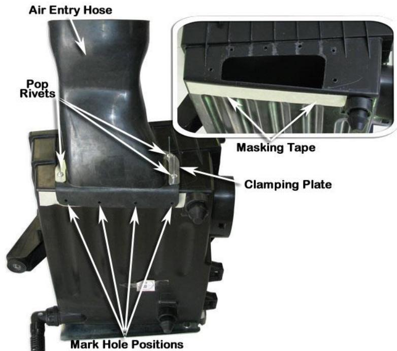
Drill a pilot hole for each of the marked hole positions.
