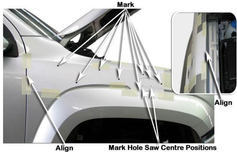
Apply masking tape to guard panel and flare to ensure no metal filings are trapped between the flare and guard panel as shown.
