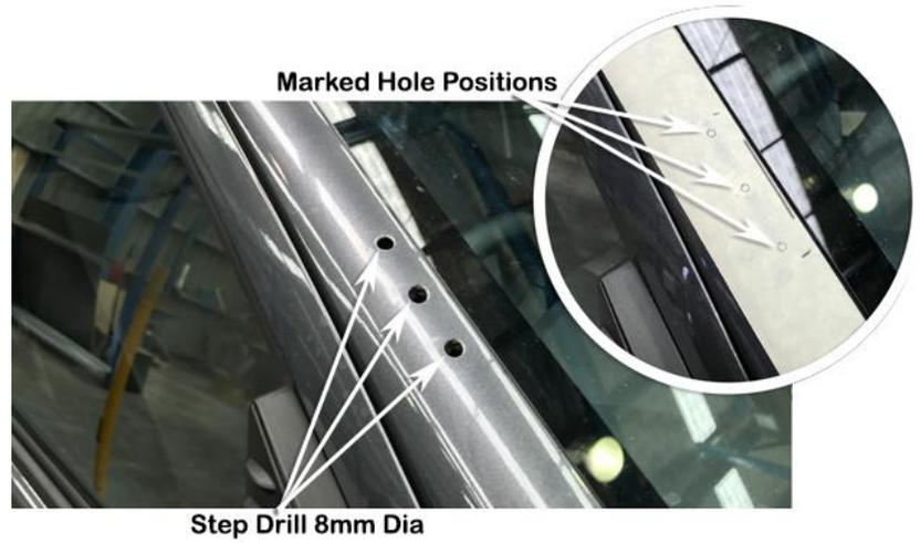
Install the plastic inserts (Item 6) into the 8mm diameter holes in the A-pillar.
