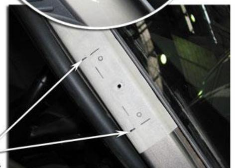
Mark the outline and the mounting hole positions of the upper mounting bracket.
