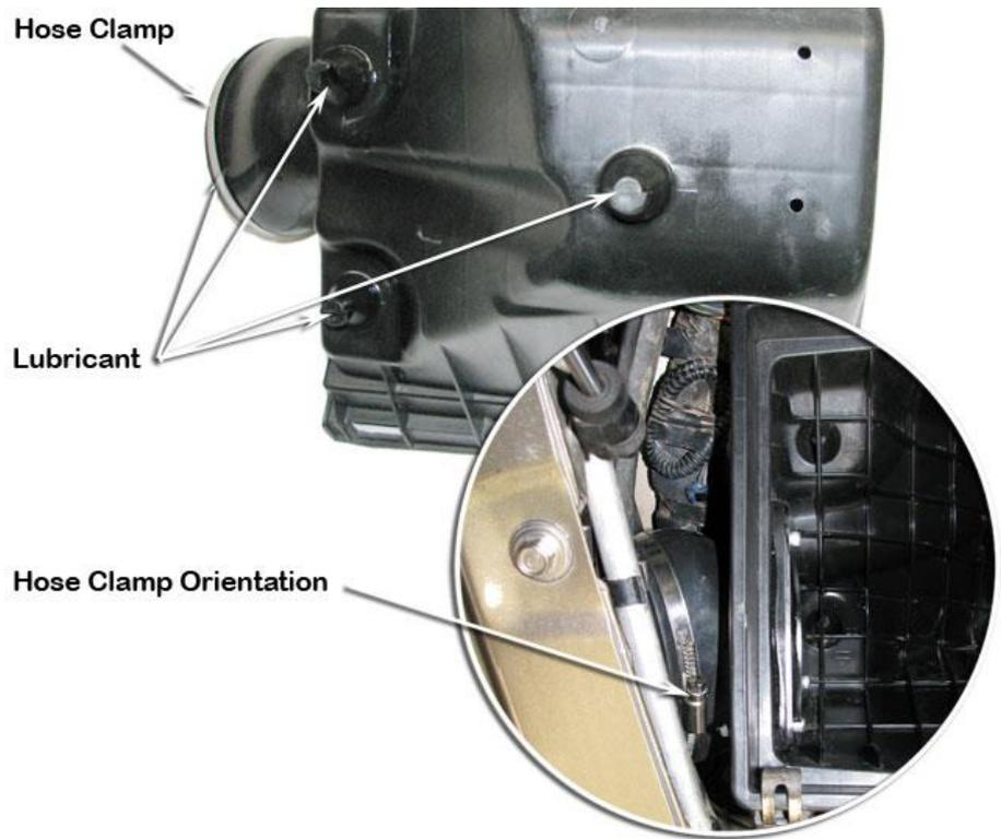
**25** Install the snorkel body (Item 1) onto the fender panel whilst guiding the snorkel body outlet into the air intake connector (Item 9).
