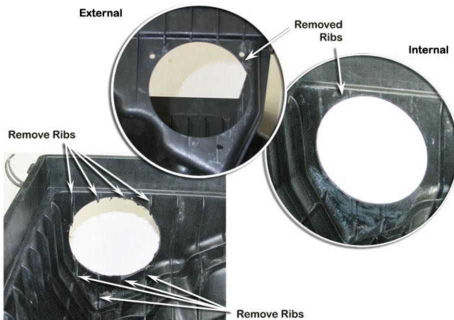
**20** Install the air intake connector (Item 9) through the 92mm hole drilled previously.
