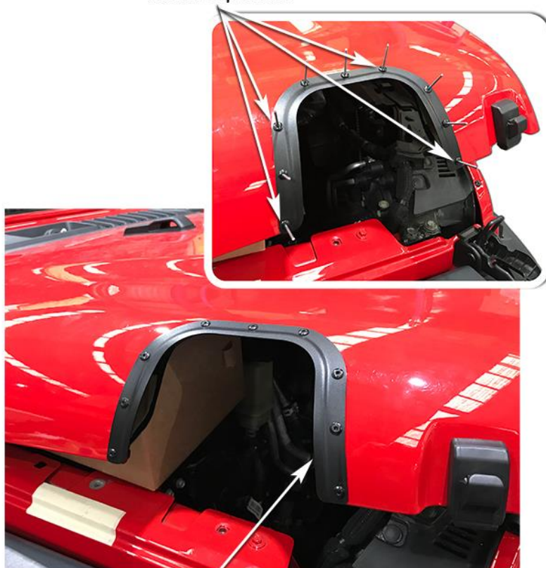
Installed Hood Bezel
