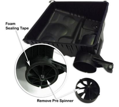
Remove the drain valve assembly from the air cleaner base.
