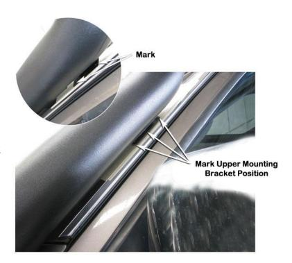
Position the upper mounting bracket onto the A-pillar and align the bracket to the scribe markings on the masking tape. Mark the three mounting hole positions with a felt tip pen.
