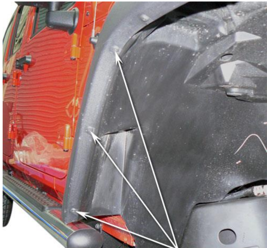
Remove Plastic Pop Rivets
