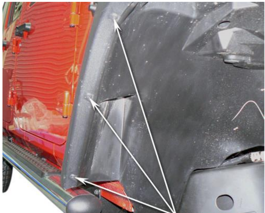
Remove Plastic Pop Rivets
