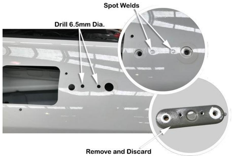
Remove and discard the perforated section of the guard panel template (item 21) as shown.
