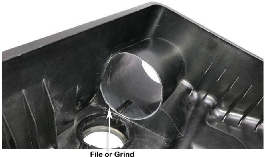
Using the body saw remove all the vanes from the pre-spinner, use a file or die grinder to remove all the remaining sections of vanes.
