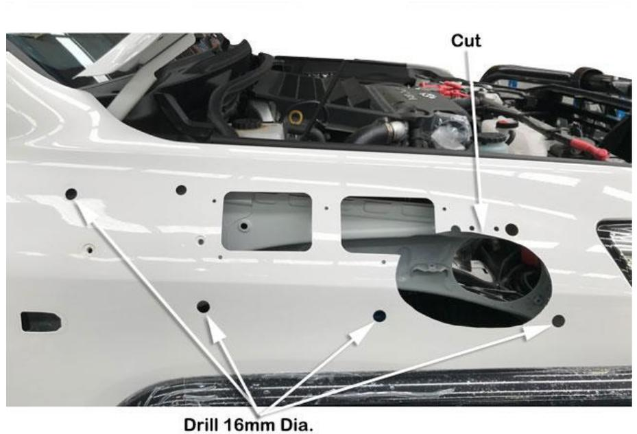
Trial fit the guard infill panel (item 14) and all five 4.8mm x 10.0mm pop rivets (item 15) to the guard panel, if necessary run the 5.5mm drill bit back through any of the holes which are not aligning up correctly to the infill panel.
