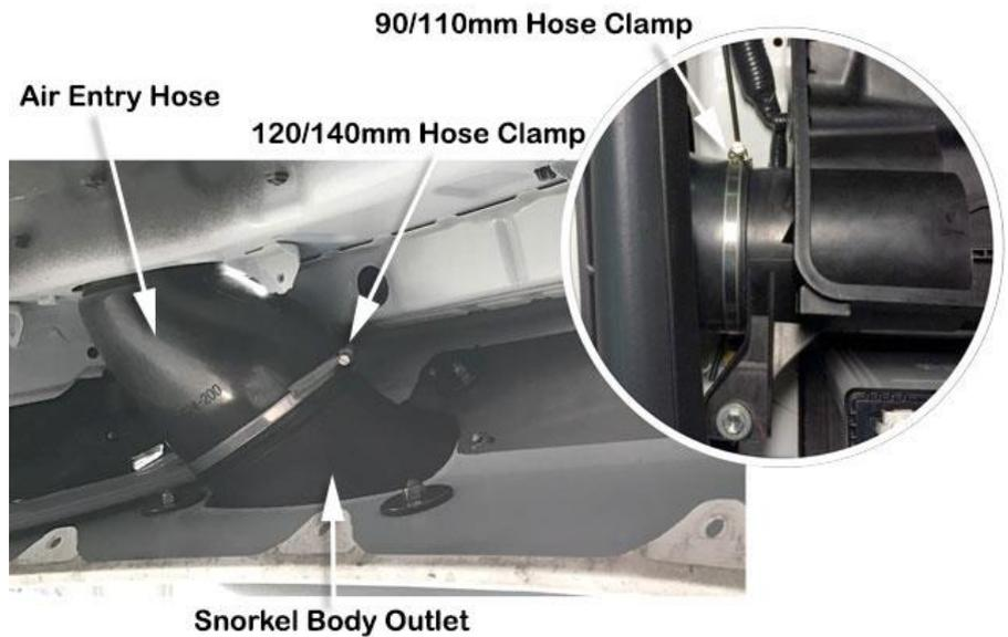
Loosely install the black hose clamp (Item 19) to the base of the air ram assembly (Item 2).
