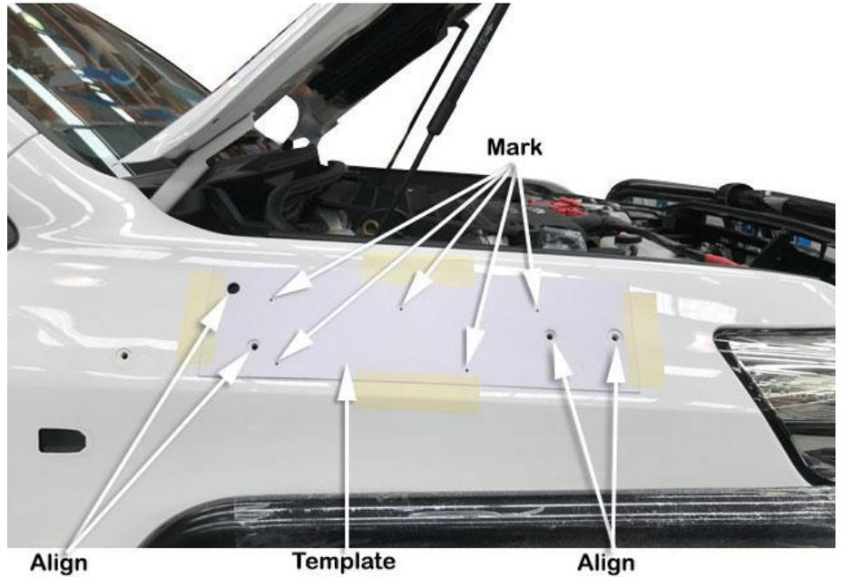
Drill a pilot hole for each of the marked hole positions, drill the five hole positions to 5.5mm diameter using a 5.5mm drill bit.
