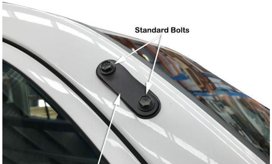
A-Pillar Blank Off Plate & Rubber Gasket
