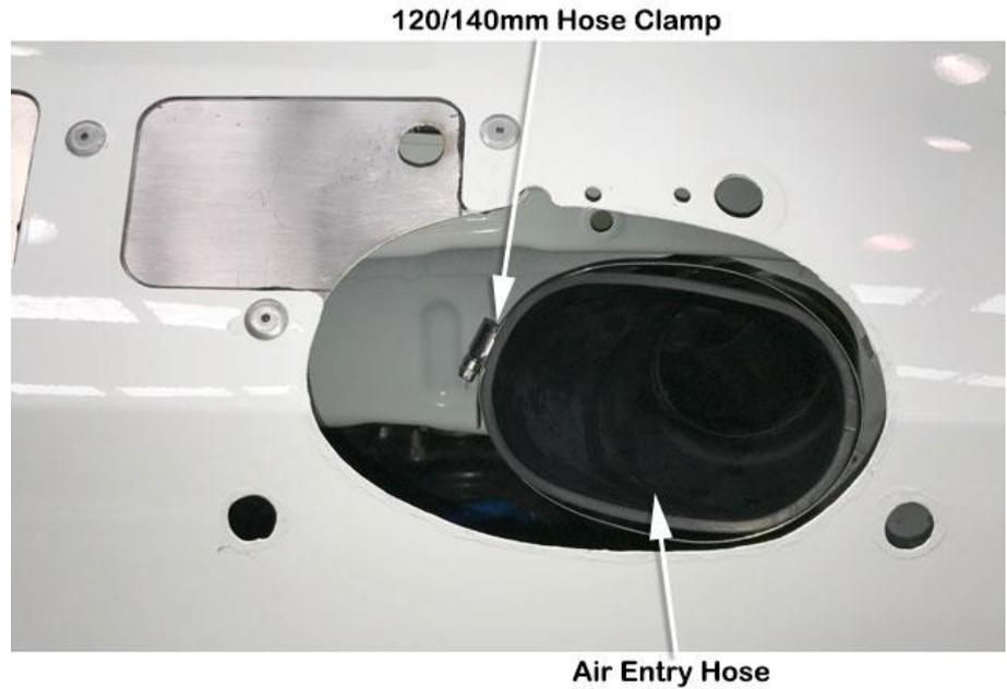
Carefully install the snorkel body (item 1) to the guard panel, guiding the snorkel body outlet snout into the air entry hose (item 11).
