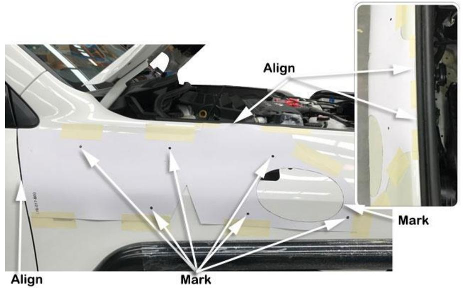
Marked mounting hole positions and guard panel cut out.
