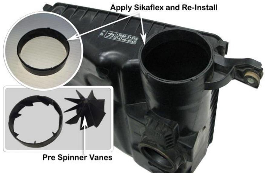
Using a scribe or paint pen, scribe or mark a line 18mm in from the end of the air cleaner inlet snout around the entire circumference as shown.
