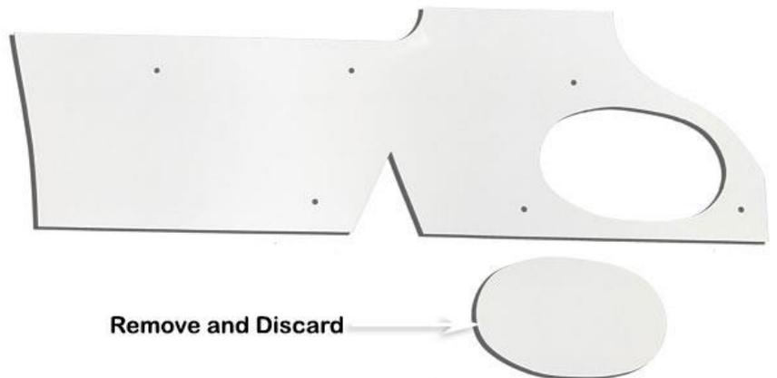
Align the guard panel template (Item 21) to the upper and rear edges of the right hand guard panel as shown.
