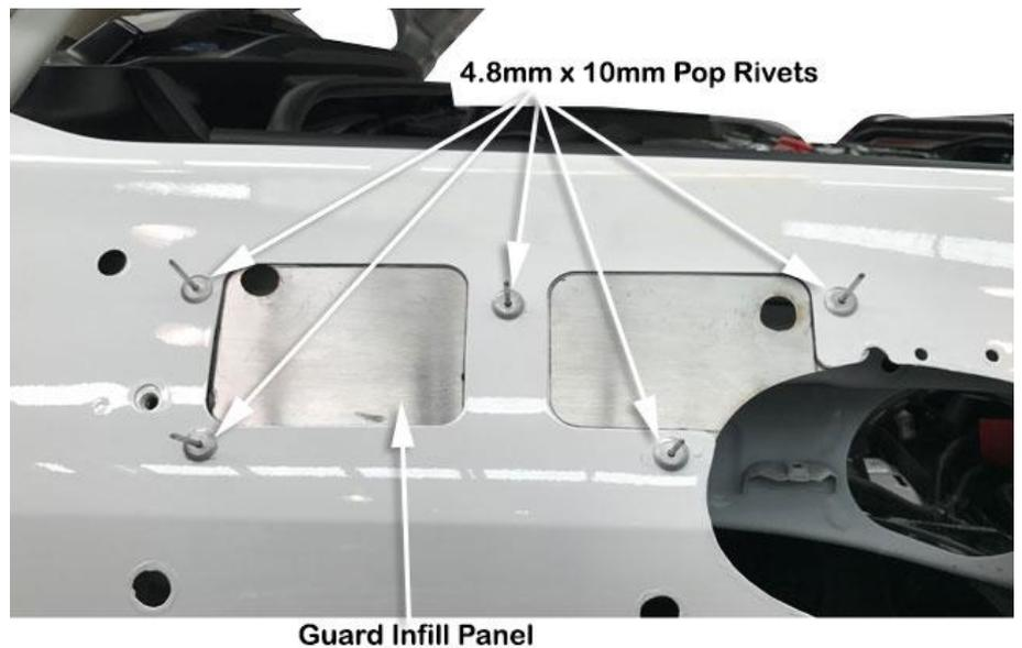
Apply Sikaflex 227 to the outer edges and centre of the guard infill panel (item 14) as shown, install the infill panel to the guard panel, install all 5 pop rivet (item 15).
