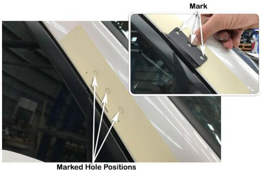
Drill a pilot hole for each of the three marked hole positions in the centre of each marked slot.
