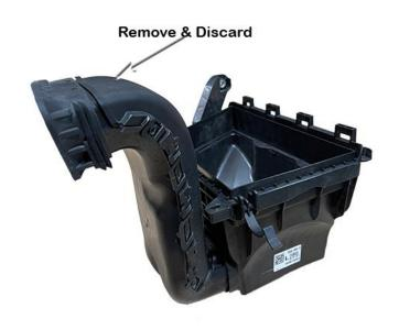
Drill a 10mm pilot hole through the air cleaner base below the 96mm diameter spigot on the side of the air cleaner base as shown.
