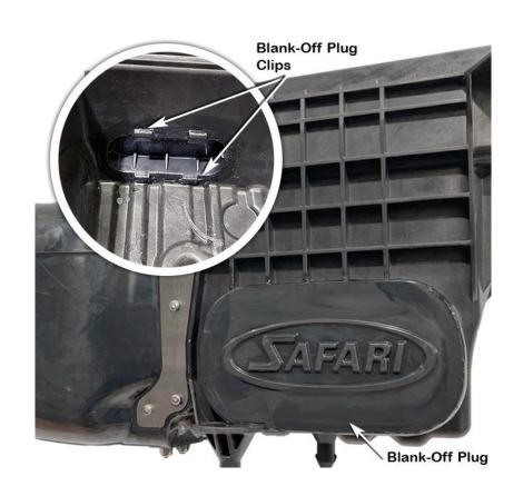
Re-install the air cleaner base into position, ensuring the mounting pins are correctly installed into the mounting grommets. Install the standard mounting bolt and fasten.
