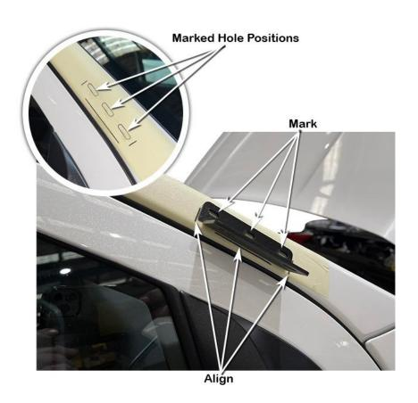
Drill a pilot hole at each of the three marked hole positions.
