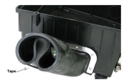
The end of the air entry hose (item 10) must be squashed inwards and taped to hold in position as shown.
