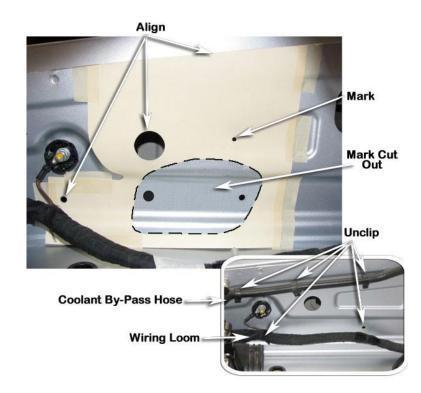
Drill a pilot hole at the marked hole position.
