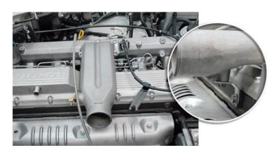
19 Install a spring hose clamp (Item 58) to each end of the 1/4" wastegate actuator hose (Item 57) and install the hose to the wastegate actuator port (Item 55).
