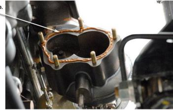
Install the turbine outlet pipe to the turbocharger outlet and retain with 8mm flat washers (Item 10) and 8mm selfloc nuts (Item 9).
