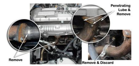
Remove the three studs shown from the exhaust manifold
