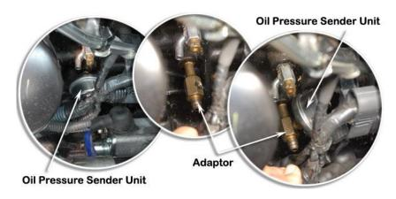
Install the 90 degree fitting end of turbocharger oil supply hose (Item 72) to the oil sender unit adaptor (Item 71).
