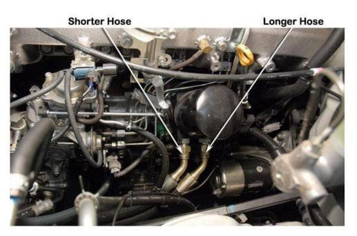
**16** Route the two hoses (Items 12 & 13) along the radiator fan shroud and over the lower radiator hose.
