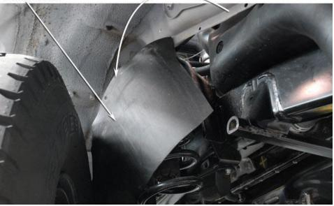
Unclip the RHS rubber inner guard liner.
