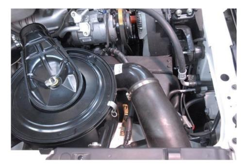
Reinstall the air cleaner assembly and secure with the original mounting hardware.
