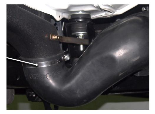
Copyright Safari 4x4 Engineering Pty Ltd Melbourne Victoria Australia – www.safari4x4.com.au Page **13** of **19**  Fit spacers (Item 43) below flange plate and bolt to front bumper support bracket (where cover was removed from) using M6 x 10 x 35mm bolts (Item 44), 6mm Star washers (Item 8) and M6 washers (Item 45).
