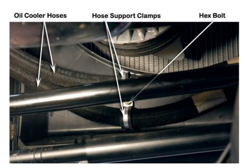
Copyright Safari 4x4 Engineering Pty Ltd Melbourne Victoria Australia – www.safari4x4.com.au Page **9** of **19**  Tighten the hose fittings at each end of the two oil cooler hoses.
