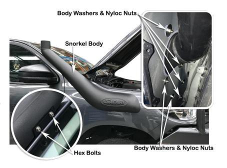
Align the air entry hose for best fitment (Ensure the air entry hose is installed hard up against the shoulder of the snorkel body outlet), correctly position the 90/110mm hose clamps at either end of the air entry hose and tighten the hose clamps.
