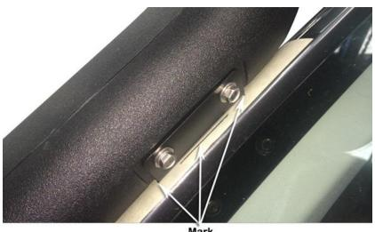
Position the upper mounting bracket (Item 3) onto the A-pillar and align the bracket with the marked bracket outline. Mark the three mounting hole positions with a felt tip pen.
