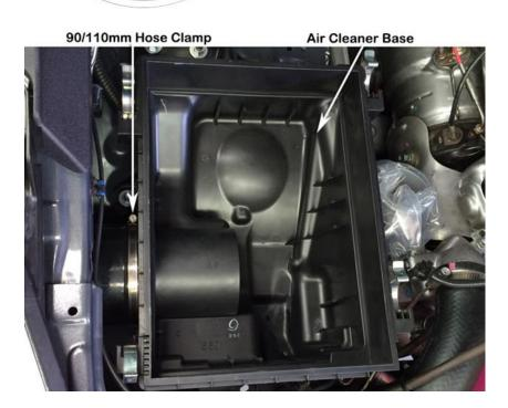
Align the air entry hose for best fitment (Ensure the air entry hose is installed hard up against the shoulder of the snorkel body outlet), correctly position the 90/110mm hose clamps at either end of the air entry hose and tighten the hose clamps.
