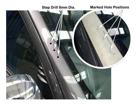
Install the plastic inserts (Item 6) into the 8mm diameter holes in the A-pillar.
