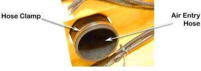
Install the modified engine air intake duct into the air entry hose (Item 10). Fasten the engine air intake duct using the stock fasteners.
