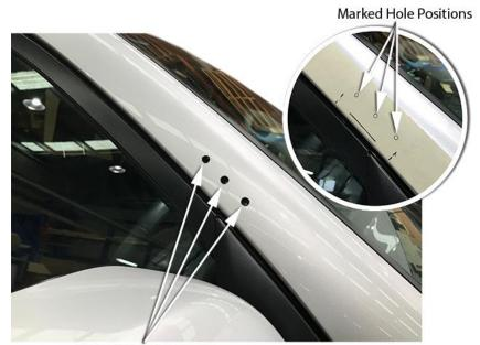
Drilled Holes 8mm Dia
