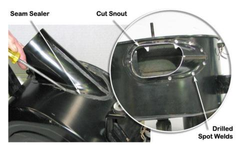
With all the spot welds drilled out use a small pry bar or flat blade screwdriver to remove the inlet snout from the air cleaner housing. Take care to avoid damaging the air cleaner housing.
