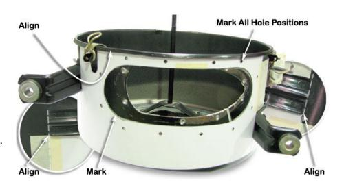
Use a 4.0mm drill bit to drill all twelve marked hole positions.
