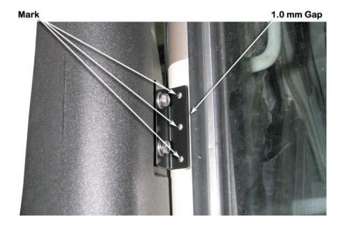
Remove the snorkel body (item 1) from the vehicle and remove the upper mounting bracket (item 3) from the snorkel body. Drill a pilot hole at each of the three marked hole positions.
