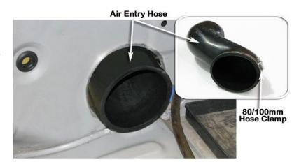
Loosely install the 60/80mm hose clamp (item 11) to the air entry hose and install the air cleaner base, fasten into position with the standard mounting bolts.
