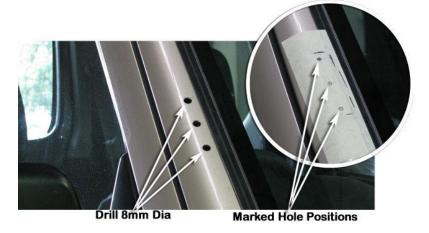
Install the plastic inserts (item 6) into the 8mm diameter holes in the A-pillar.
