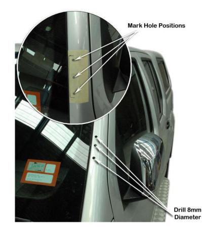
Install the plastic inserts (Item 6) into the 8mm diameter holes in the Apillar.
