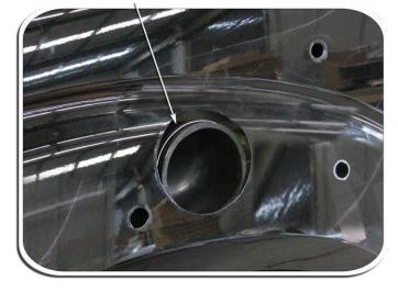
Carefully install the snorkel body (item 1) to the guard panel, guiding the snorkel body outlet snout into the air entry hose (item 10), align the snorkel body to the guard panel and upper mounting bracket.
