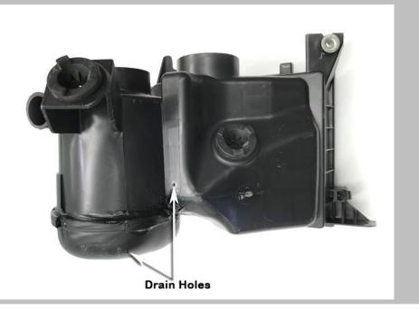
The air inlet duct is a two piece part which must be sealed correctly to prevent water from entering the air intake of the vehicle. Apply a generous amount of adhesive sealant to the upper and lower joins of the air inlet duct, ensure both sides are completely sealed as shown.
