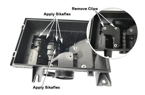
The air cleaner base has areas which are not totally sealed in various positions, apply a generous amount of Sikaflex to the unsealed areas of the air cleaner base as shown.
