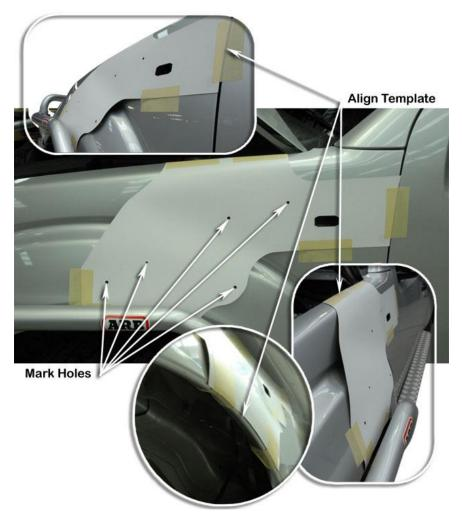
Drill a pilot hole for each marked hole position. Using the 105mm hole saw, drill the main hole in the guard panel. Using the step drill, drill the 4 mounting hole positions to 16mm.
