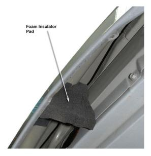
Remove and discard the foam insulator from between the inner and outer guard panel.
