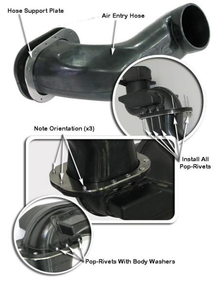
The air inlet duct is a two piece part which must be sealed correctly to prevent water from entering the air intake of the vehicle. Apply a generous amount of adhesive sealant to the joins, upper and lower chambers of the air inlet duct, ensure the duct is completely sealed.
