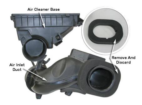
Remove the air inlet duct from the air cleaner housing base by rotating the air inlet duct in an anti-clockwise direction.
