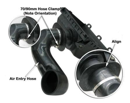
Apply CRC 5.56 multipurpose lubricant or similar lubricant to the outer surface of the air entry hose (item 10).
