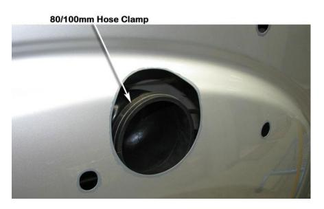
Carefully install the snorkel body (item 1) to the guard panel, guiding the snorkel body outlet snout into the air entry hose (item 10), align the snorkel body to the guard panel and upper mounting bracket.
