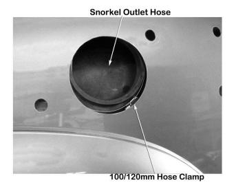
Carefully install the snorkel body (item 1) to the guard panel guiding the snorkel body outlet snout into the snorkel outlet hose (item 10), align the snorkel body to the guard panel and upper mounting bracket.
