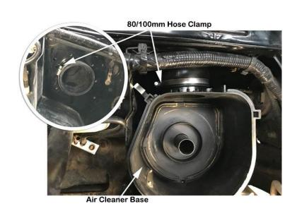
Loosely install the 80/100mm hose clamp (item 13) over the snorkel outlet hose (item 10), install the hose onto the joiner, loosely install a 90/110mm hose clamp to the snorkel body outlet end of the hose and align the hose with the hole in the guard panel.
