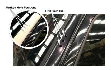
Install the plastic inserts (item 6) into the 8mm diameter holes in the A-pillar.
