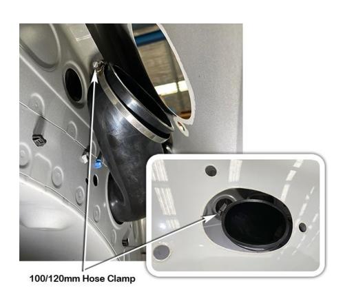
When correctly aligned, fasten the snorkel body to the guard panel with body washers (Item 8) and nyloc nuts (Item 9).
