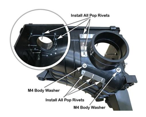
With the air entry hose, pop rivets and hose support plates correctly installed, secure all the pop rivets using a pop rivet gun.
