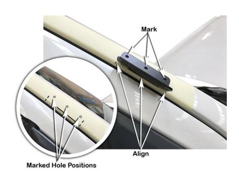
Drill a pilot hole at each of the three marked hole positions. Drill each hole position to 8mm diameter with a step drill or 8mm drill bit.
