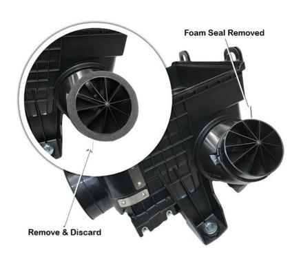
The standard air cleaner base inlet must be sealed by the installer.
