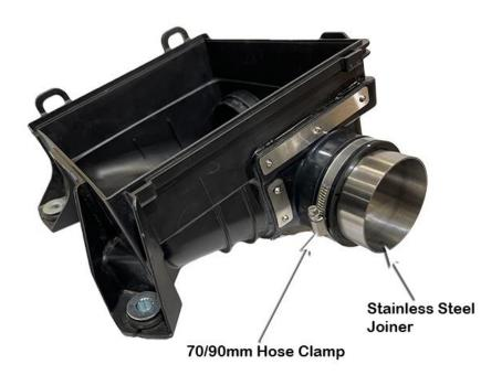
Install the snorkel outlet hose (Item 10) through the hole in the inner guard panel, loosely install a 70/90mm hose clamp (item 21) onto the hose and install the snorkel outlet hose onto the stainless steel joiner (item 12).
