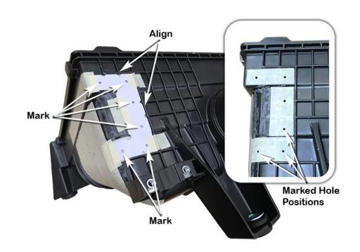
Drill a pilot hole for each of the seventeen marked hole positions, drill each hole position to 4.5mm diameter with a 4.5mm drill bit.
