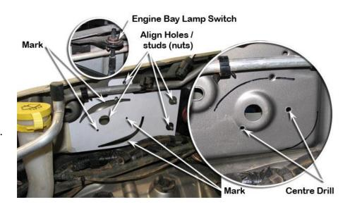
Use a 76mm diameter hole saw and drill the two hole positions.
