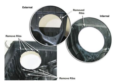
20 Install the air intake connector (Item 9) through the 92mm hole drilled previously.
