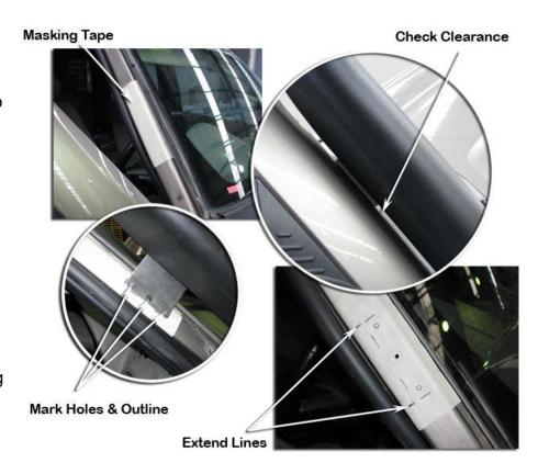
Mark the outline and the mounting hole positions of the upper mounting bracket. Remove the snorkel body and extend the outline marked lines as shown.
